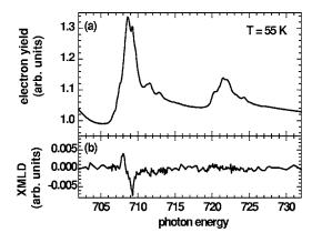
FIG. 3. (a) Fe  $L_{3,2}$  spectrum measured in normal incidence with linearly polarized x-rays at T=55 K. The average of spectra obtained with the polarization axis parallel and perpendicular to the FeF<sub>2</sub>(001) direction is shown. (b) XMLD spectrum; that is, the difference of the spectra observed in normal incidence by switching a magnetic field of 0.65 T in the sample plane between parallel and perpendicular to the polarization axis of the linearly polarized x rays.
