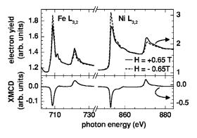
FIG. 1. (a) Fe and Ni  $L_{3,2}$  spectra of a 20 Å Ni/500 Å FeF<sub>2</sub> bilayer measured at T=55 K. Spectra obtained for parallel and antiparallel orientation of external field and photon helicity are indicated by a dotted and a solid line, respectively. (b) XMCD spectrum of the same sample, that is, the difference of the spectra shown in (a).
