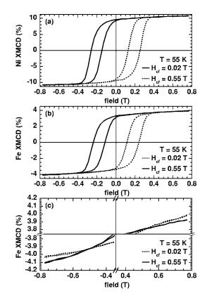
FIG. 2. Hysteresis loops measured at the (a) Ni and (b) Fe L edges after cooling the sample in fields of  $H_{cf}$ =0.02 T (solid line) and  $H_{cf}$ =0.55 T (dotted line) to 55 K. A magnified view of (b) at high fields is shown in (c).
